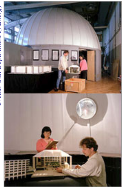
This sky simulator provides a test facility for researchers and building design professionals to conduct model studies on daylighting.
