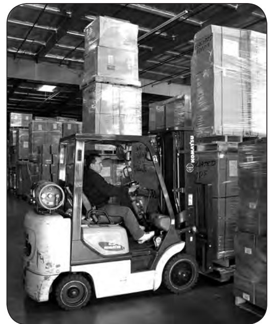
This forklift is fueled by propane.
