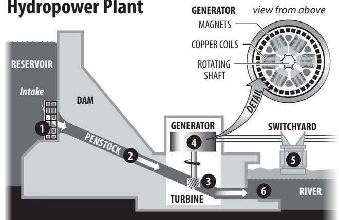
1. Water in a reservoir behind a hydropower dam flows through an intake screen, which filters out large debris, but allows fish to pass through.
