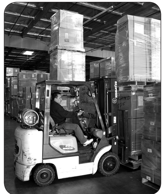
This forklift is fueled by propane.
