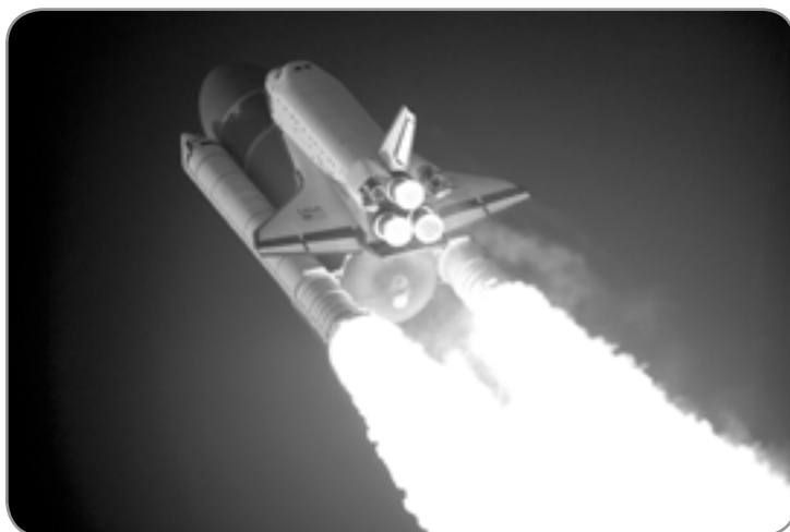
NASA once used hydrogen to fuel the space shuttle. Hydrogen batteries—called fuel cells —powered the shuttle's electrical systems.
