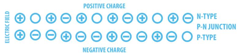
**3** If the PV cell is placed in the sun, photons of light strike the electrons in the p-n junction and energize them, knocking them free of their atoms. These electrons are attracted to the positive charge in the n-type silicon and repelled by the negative charge in the p-type silicon. Most photon-electron collisions actually occur in the silicon base.
