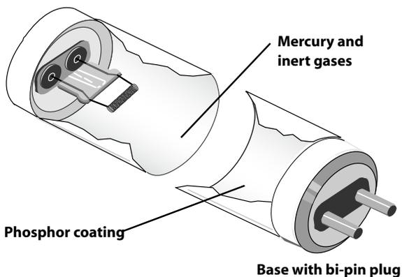
In fluorescent tubes, a very small amount of mercury mixes with inert gases to conduct the electrical current. This allows the phosphor coating on the glass tube to emit light.
