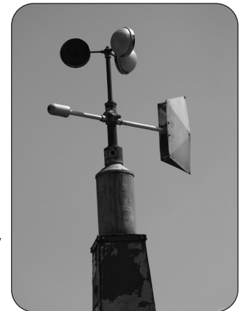
An anemometer and wind vane combined in one tool.
