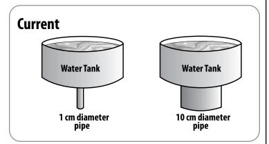
two points having a difference in voltage. Current is measured in **amperes** or **amps (A)**. One ampere is 6.25 X 10<sup>18</sup> electrons per second passing through a circuit.
