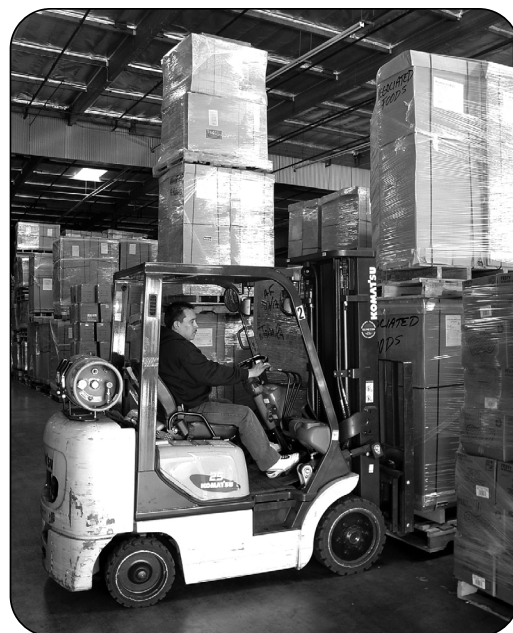
This forklift is fueled by propane.
